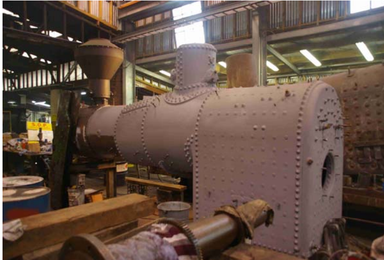
Climax Boiler from 1694 ready to steam Belgrave Workshops 10 July 2009
